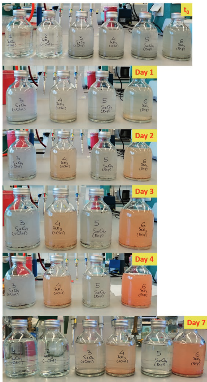
Fig. 2 Anaerobic incubation using granular sludge and selenium oxyanions. (1) Abiotic control [10 mM \text{SeO}_4^{2-} and 10 mM lactate], (2) abiotic control [10 mM \text{SeO}_3^{2-} and 10 mM lactate], (3) [10 mM \text{SeO}_4^{2-} without electron donor + granular sludge], (4) [10 mM \text{SeO}_3^{2-} without electron donor + granular sludge], (5) [10 mM \text{SeO}_4^{2-} and 10 mM lactate + granular sludge], and (6) [10 mM \text{SeO}_3^{2-} and 10 mM lactate + granular sludge]. Abiotic controls: 1 and 2; biotic incubations: 2–6
