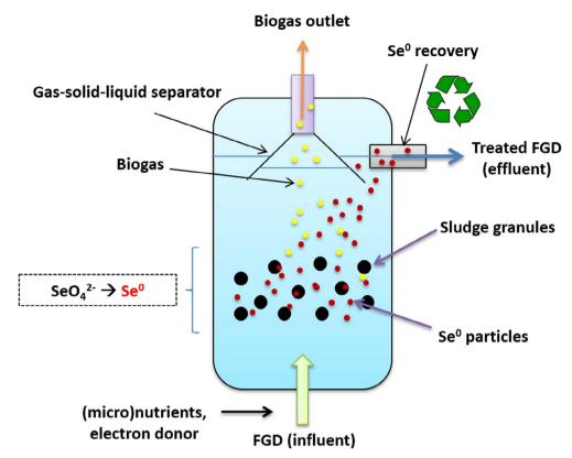
Fig. 4. Bioremediation of selenium-containing industrial effluents using an UASB system.
