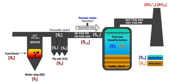
Fig. 1. Diagram of a coal-fired power plant equipped with a flue gas desulfurization (FGD) system. Legend: S<sub>i</sub> to S<sub>m</sub> refers to the partitioning of a given element in the *in* and *outgoing* streams during PCC-FGD process.
