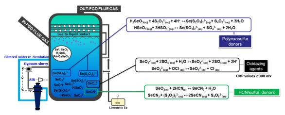
Fig. 2. Selenium chemistry in wet limestone FGD systems.
